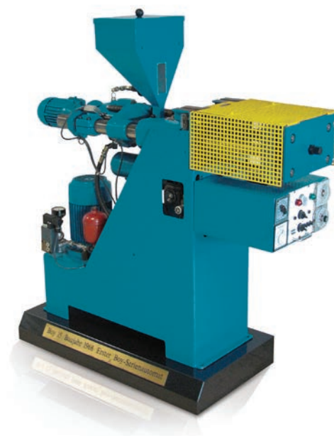
BOY 15 – worldwide the first injection moulding machine with the fully hydraulic, two-platen clamping system, from 1968.
