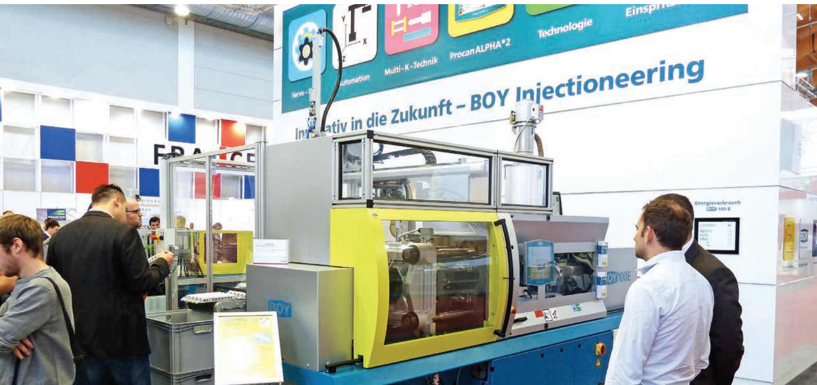
A complete manufacturing system: Injection moulding machine BOY 100 E with four-axis industrial robot handling LR 5, as well as a protective enclosure conforming to CE.
