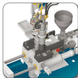
Injection unit in slidable vertical position on top of the fixed platen
